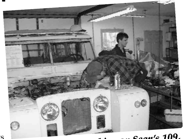
▲ Jeff and John working on Sean's 109, a IIA in for a conversion from diesel to gas.
